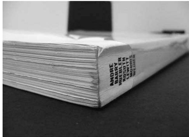
Detail of the original flat-back adhesive binding.
